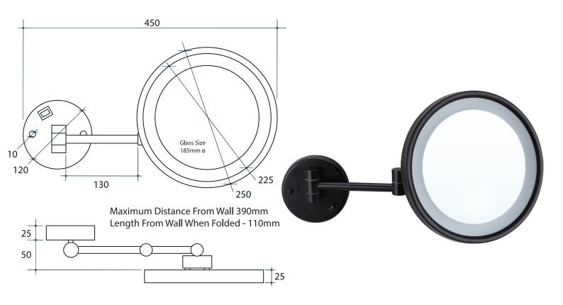
Note: All dimensions are in millimetres (mm)
