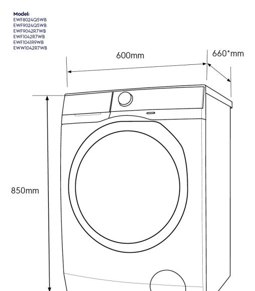
\*Add 20mm for the hose protrusion at the back.
