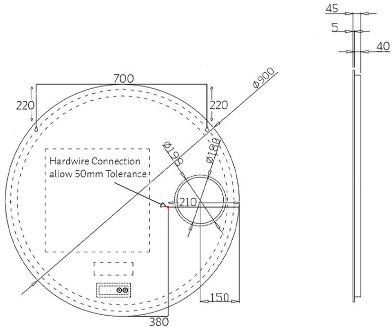
Note: All dimensions are in millimetres and are subject to normal manufacturing variations. Always use the physical product measurements for cut-outs and rough-ins as the technical details shown may differ from the actual product. Use acetic cured silicone sealant. Do not use epoxy type adhesives. Clean with damp cloth. Do not use abrasive cleaners, liquids or pastes.
