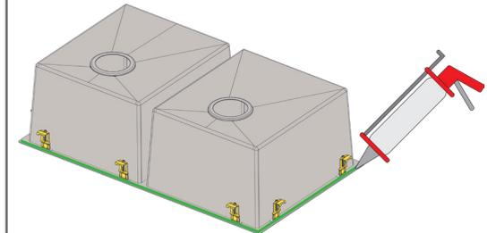
Apply adhesive sealant under the sink to ensure a tight seal. **DO NOT USE EPOXY.**
