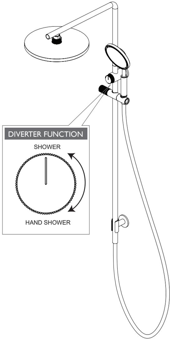
**1** Position Diverter Body in preferred location. Ensure Rail is level and mark positions of holes.
