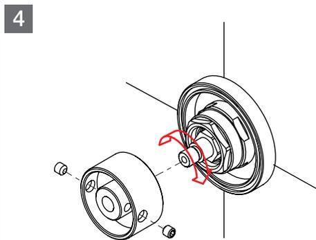
Turn the spindle clockwise until the cartridge is set to OFF position. Fit the spindle adaptor to the spindle. Secure it with the two grub screws as shown.
