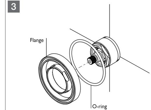
Ensure the o-ring is seated in the flange. Screw the flange onto the bonnet until it sits hard up against the finished wall surface.
