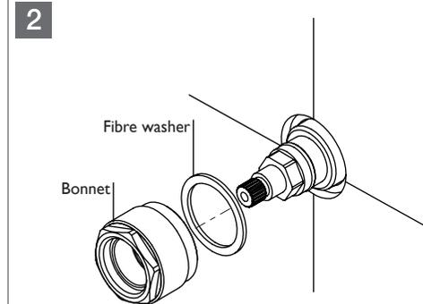
Fit the fibre washer over the spindle and then fasten the bonnet onto the spindle using a spanner.
