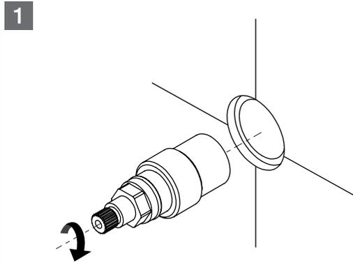
Firmly screw the spindle into the breach.
