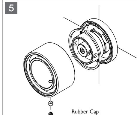
Fit the washer into the groove on the flange. Place the handle onto the spindle adaptor and secure it with the grub screw. Fit Rubber Cap to position.
