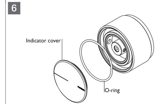
Ensure the o-ring is seated on the indicator cover. Apply some grease or soapy water to O-Ring if necessary. Push the indicator cover into the handle.
