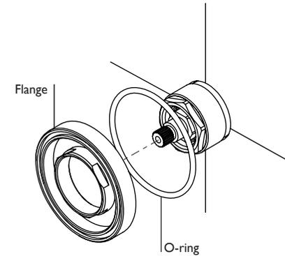
**3** Turn the spindle clockwise until the cartridge is set to OFF position.
