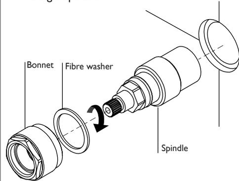
**2** Ensure the o-ring is seated in the flange.
