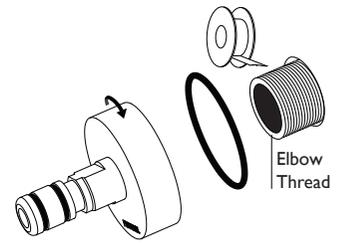
**4** Fit O-Ring to the base of the handle assembly.
