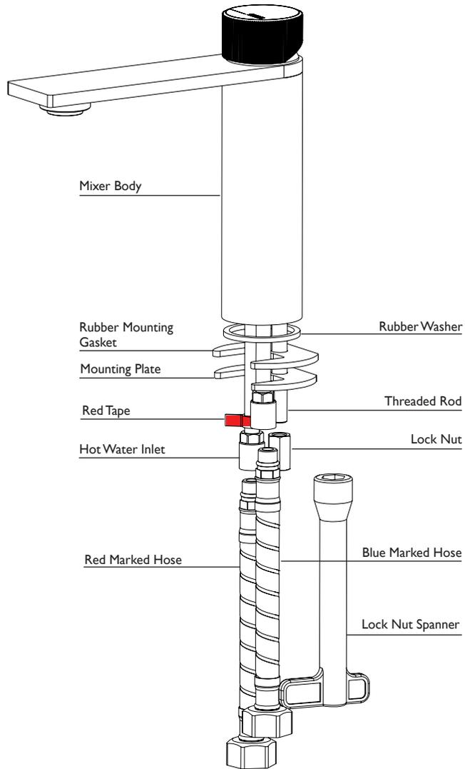
**1** Cut a mounting hole 35mm in diameter. There must be a minimum 12mm clearance around the hole.
