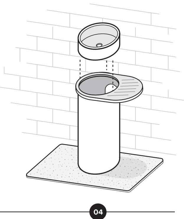
Place sink carefully onto ring of tray. Fix basin down with screws (from access hole beneath).
