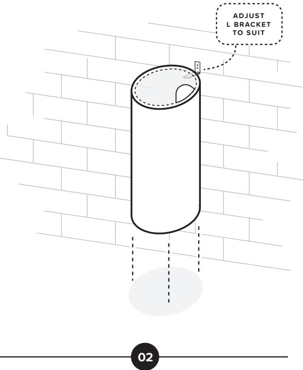
Place cylinder in position with access hole reachable. Adjust feet at bottom to level. Adjust L bracket to suit.
