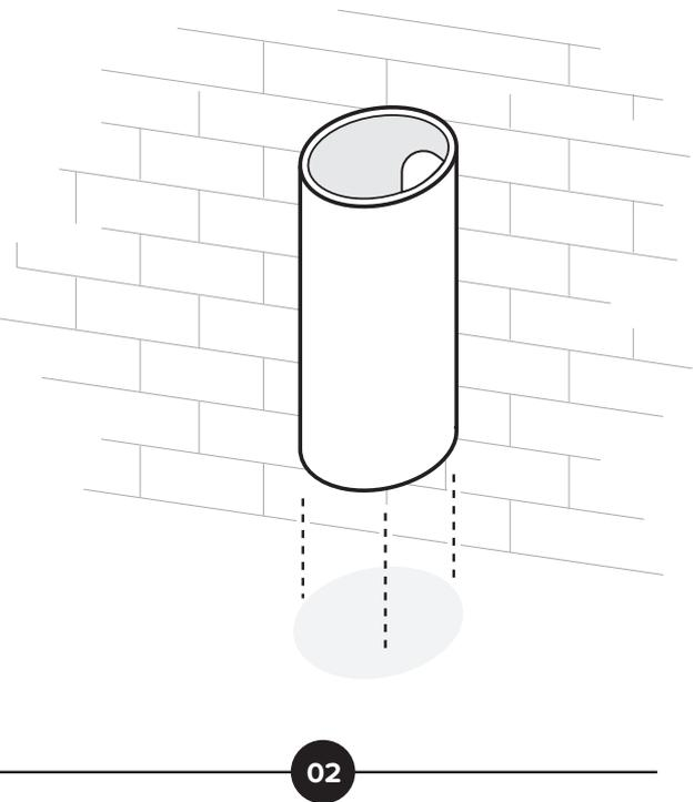
Place cylinder in position. Adjust feet at bottom to level. Adjust L bracket to suit.
