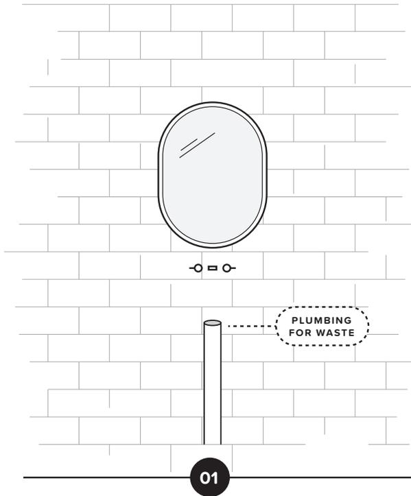
Ensure plumbing for waste is in place, either wall or floor.
