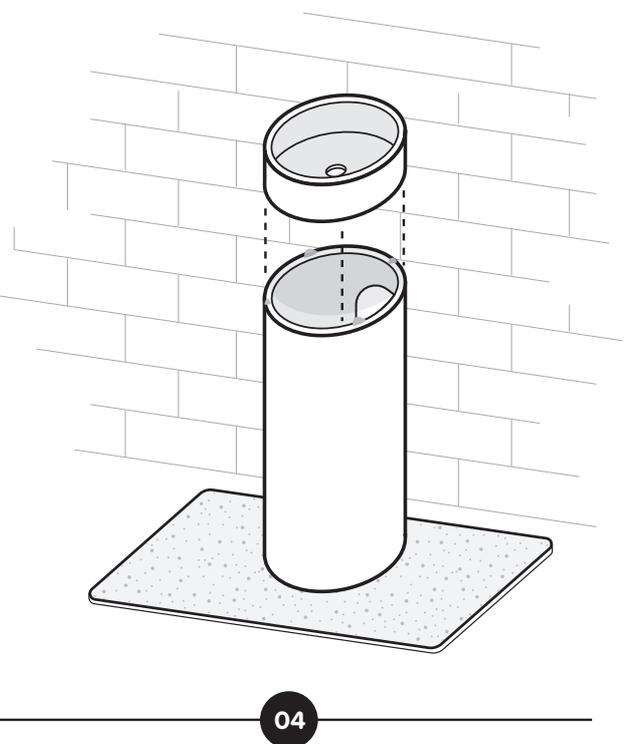
Place sink carefully and line up holes of both plates. Use screws to tighten from underneath.
