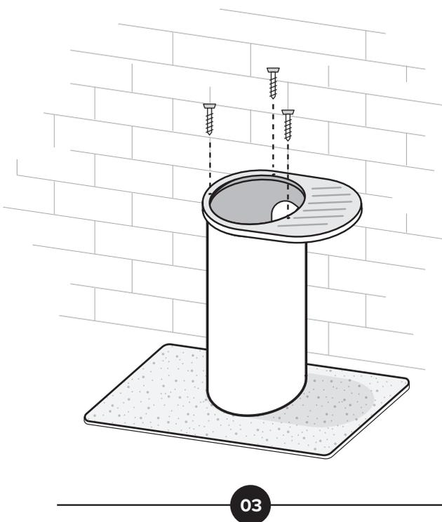
Ensure hand can reach access hole. Fix down from the top with screws provided.
