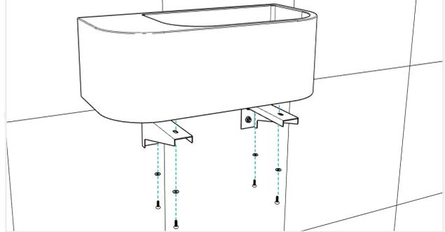
3. Hold the basin against the wall in the desired position according to the centre line and adjust to be flat and centred. Mark the position of the bracket fixing holes onto the wall. Remove the basin and drill four holes in the masonry wall using a 10mm masonry drill bit, to the required depth.
