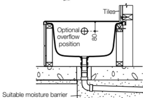
Under-rim support suitable for built-in installations. The Stirling bath is not suitable for island installations
