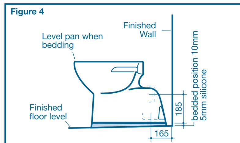
**IMPORTANT:** ALL DIMENSIONS ARE TO THE UNDERSIDE FOOTLEVEL OF THE PAN. IT IS IMPORTANT TO MAKE A HEIGHT ALLOWANCE FOR BEDDING.
