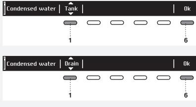
Press the button 1 for to appear. Use the program selector knob or the button 1 to choose between following: "Tank" – run condensate water into a condensate tank
