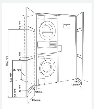
$\overline{\ }$  Ensure the dryer door can be opened without hindrance after installation.
