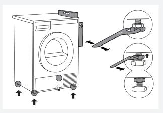
Place the dryer so that it is stable. Use a spirit level to level the dryer in longitudinal and traverse direction by rotating the adjustable feet using a No. 22 spanner (max. 15 mm). Then, firmly tighten the jam nuts (counter nuts) by rotating them towards the appliance bottom using a No. 17 spanner **1**.
