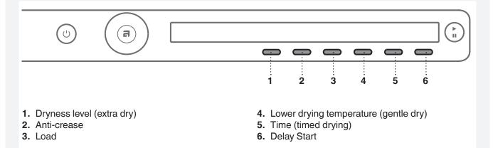
Choose the program settings before pressing the START button. When the drying program is in progress, program settings cannot be changed.
