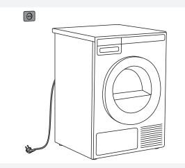
$\dot{\dot{\phi}}$  Always disconnect the dryer from the power mains before cleaning.
