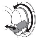
If necessary, clean the filter housing and door gasket as well.
