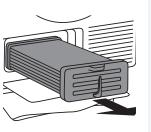
Rotate the condenser unit lever up. Use the handle to pull out the condenser unit.
