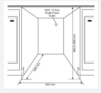
ASKO dryers can be installed beneath a cabinet or worktop with a minimum height of 864 mm. There must be a gap of about 12 mm all around the machine and a minimum gap of 25 mm between the rear edge of the machine top panel and the back wall. The opening width must be at least 622 mm. The condensing models work best when they have good air circulation.
