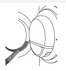
Opening on the lower side of the door should occasionally be cleaned with a vacuum cleaner.
