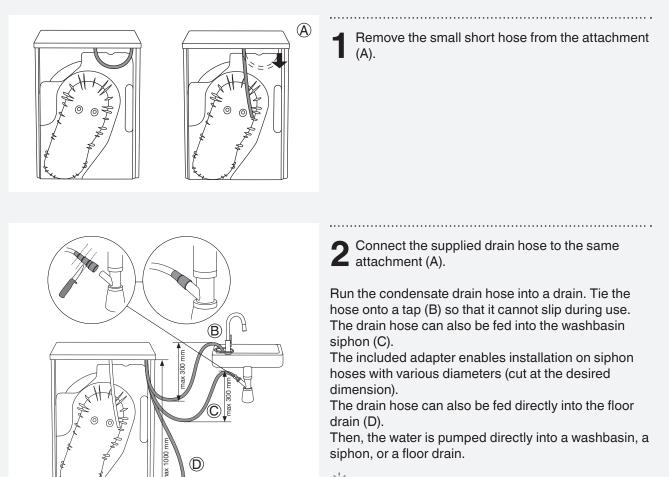
$\dot{\dot{V}}$  Do not pull the drain hose, and make sure it is not under tension, clamped, or bent.
