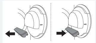
If you have inadvertently removed the **entire** net filter housing in the dryer door, reinstall it in the same position.
