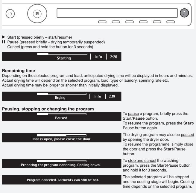
Only after the cooling is complete, can you use the program selector knob to select a new program and press the **Start**/Pause button.
