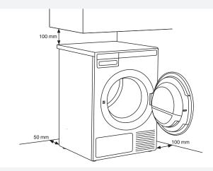
$\overline{O}^{-1}$  The appliance shall not be in contact with a wall or adjacent furniture. For optimum operation of the drying machine, it is recommended to consider the deviation from the wall, as shown in picture.
