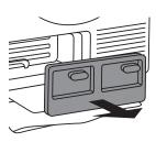
**2** Hold the levers on the inside cover and rotate them upwards. Remove the inside cover.
