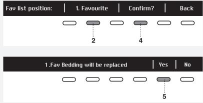
Use the button 2 to scroll through the list of Favourite programs. Press the button 4 to confirm the program to be replaced.
