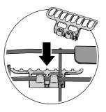
Fit the cutlery holder to achieve maximum loading capacity. (Found inside the enclosed plastic bag.)
