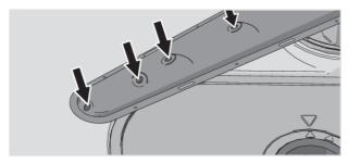
To facilitate cleaning, you can remove the spray arms. Remember to fit them firmly back into place after cleaning.
