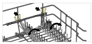
At the back of the right side of the lower basket, the plate supports can be pushed together to provide more space, for example for stoneware or a deep pan.
