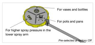
Leave the power zones open if you want an increased water flow, for example where you have placed pots and pans or vases and bottles. Turn the dishwasher's power zones off if you want greater spray pressure in the lower spray arm.
