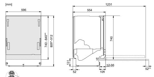
\*Remove the locking nuts when installing in a recess measuring 860-861 mm.
