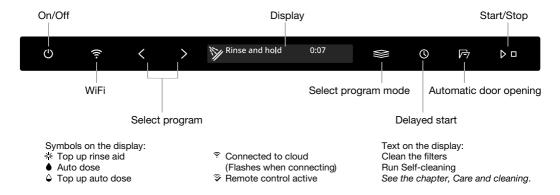
To install the dishwasher see the chapter, *Installation*. Then open the door and press  $\circ$ .
