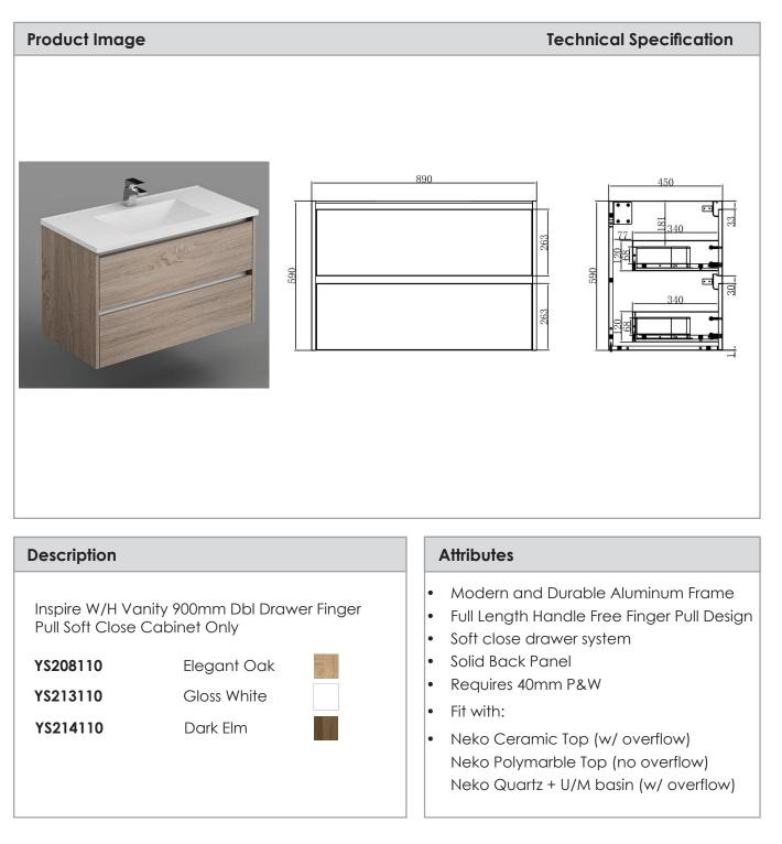
\*All dimensions are in millimeters and are subject to normal manufacturing variations. Actual dimensions should be checked prior to installation. Yushi pursues a policy of continuing improvement in design and performance of its products. The right is therefore reserved to vary specifications without notice.
