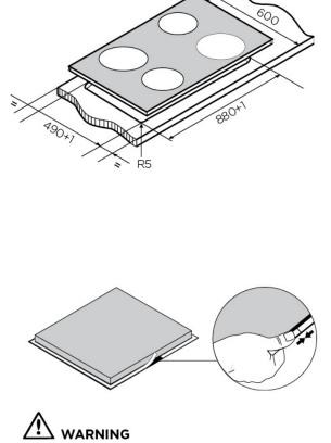
Surface temperatures of base exceed 95°C, under bench access must be restricted by use of non-combustible barrier on installation
