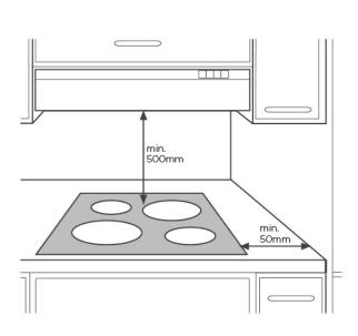
NOTE: The clearance must meet or exceed the minimum recommended for both the rangehood and cooktop. Refer to the rangehood installation manual.
