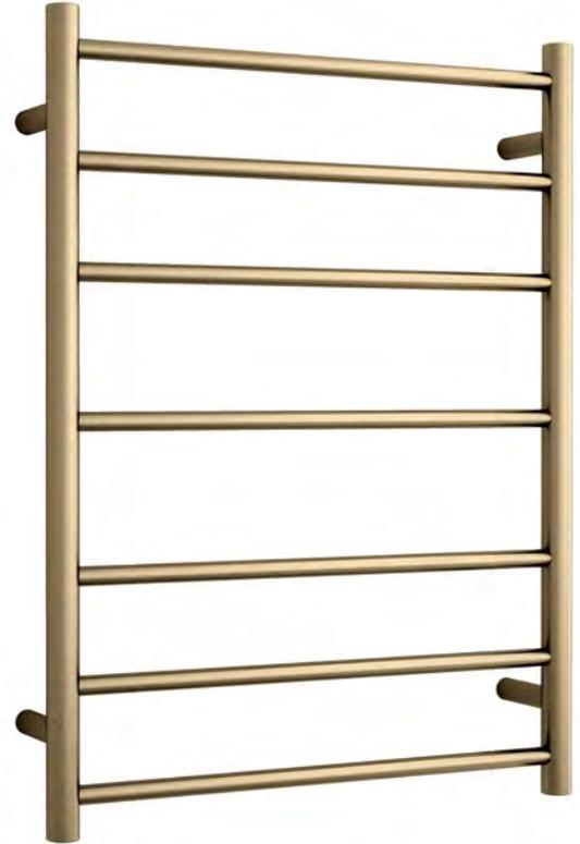
This rail has Multiflex wiring which means that there is a connection point on both the left and right hand side of the rail and the lead can be connected to either side. Being a dry element rail, this can be mounted either way up meaning the wiring can be from any of the four mounting points.
