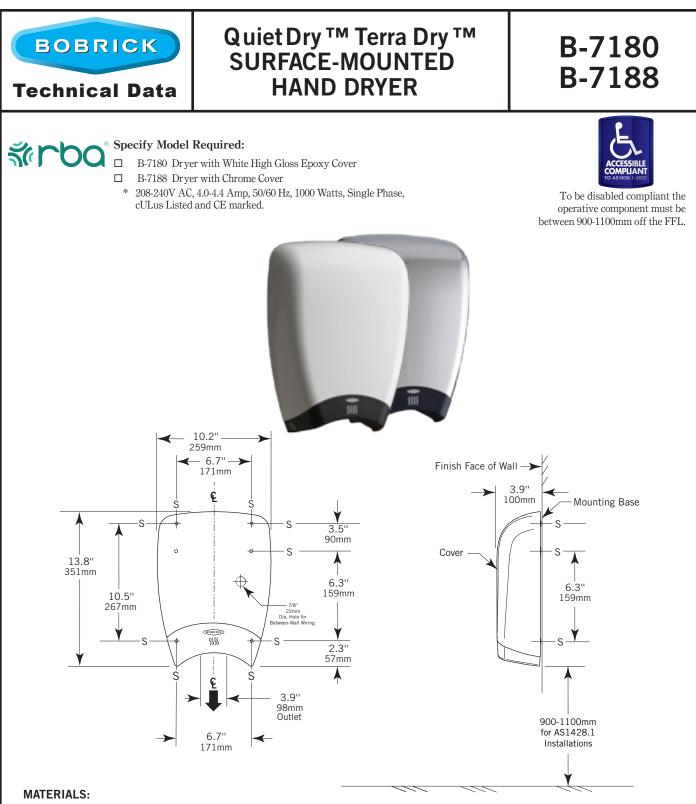
**Cover** — Aluminum die-casting with high-gloss epoxy finish electrostatically applied. White (B-7180) and Chrome (B-7188). Cover projects no more than 4" (100mm) from wall and is secured to mounting base with two vandal-resistant, recessed hex-screws.
