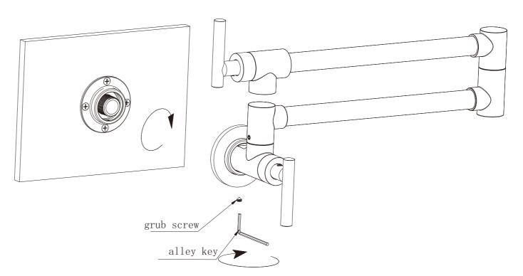
3. Screw pot filler onto outlet thread and tight it firmly by grub screws.
