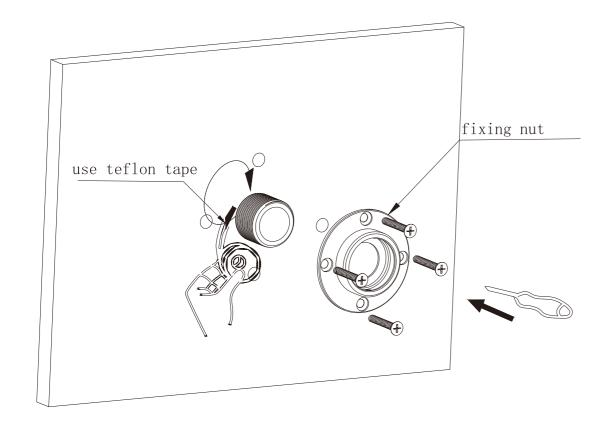
2. Put teflon tape onto outlet thread, then screw fixing nut onto outlet thread and tight it firmly by 4 screws.
