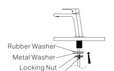
3. Install the rubber and metal washers, tighten the locking nut securely with the two M6 screws to ensure the mixer is firmly attached to the counter-top.
