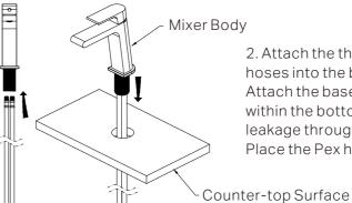
2. Attach the threaded tube to mixer body and screw the Pex hoses into the bottom of the mixer body.
