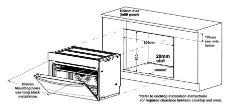
NOTE: If a powerpoint is fitted it must be accessible with the appliance installed.
