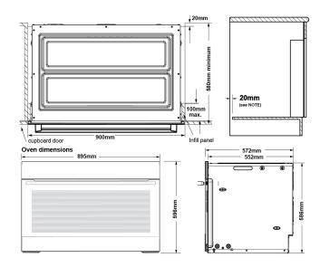
NOTE: If a powerpoint is fitted it must be accessible with the appliance installed.
