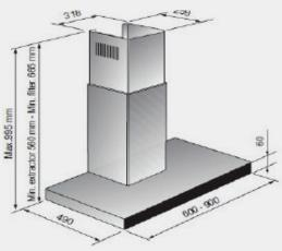
Method of installation: Can be ducted or recirculated Dimensions: 900W x 490D x 60Hmm
