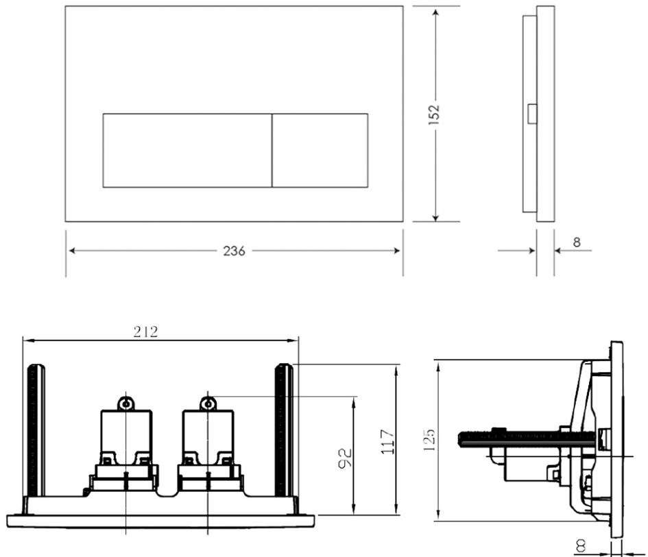
Note: All dimensions are in millimetres and are subject to normal manufacturing variations. Always use the physical product measurements for cut-outs and rough-ins as the technical details shown may differ from the actual product. Use acetic cured silicone sealant. Do not use epoxy type adhesives. Clean with damp cloth. Do not use abrasive cleaners, liquids or pastes.
