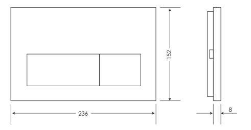
Note: All dimensions are in millimetres and are subject to normal manufacturing variations. Always use the physical product measurements for cut-outs and rough-ins as the technical details shown may differ from the actual product. Use acetic cured silicone sealant. Do not use epoxy type adhesives. Clean with damp cloth. Do not use abrasive cleaners, liquids or pastes.
