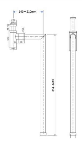
Note: All dimensions are in millimetres and are subject to normal manufacturing variations. Always use the physical product measurements for cut-outs and rough-ins as the technical details shown may differ from the actual product. Use acetic cured silicone sealant. Do not use epoxy type adhesives. Clean with damp cloth. Do not use abrasive cleaners, liquids or pastes.
