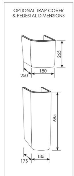
Note: All dimensions are in millimetres and are subject to normal manufacturing variations. Always use the physical product measurements for cut-outs and rough-ins as the technical details shown may differ from the actual product. Use acetic cured silicone sealant. Do not use epoxy type adhesives. Clean with damp cloth. Do not use abrasive cleaners, liquids or pastes.
