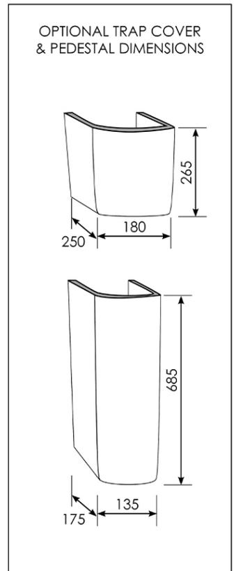
*Note: All dimensions are in millimetres and are subject to normal manufacturing variations. Always use the physical product measurements for cut-outs and rough-ins as the technical details shown may differ from the actual product. Use acetic cured silicone sealant. Do not use epoxy type adhesives. Clean with damp cloth. Do not use abrasive cleaners, liquids or pastes.*
